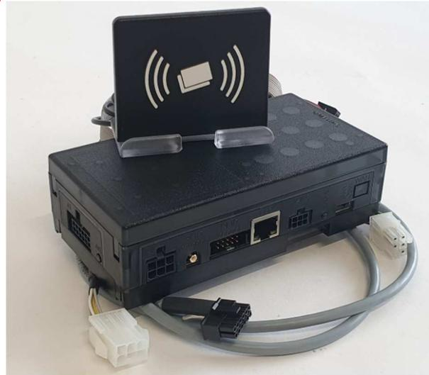
Various antennas accept all common transponders for hands free operation and can be easily installed in any machine.
